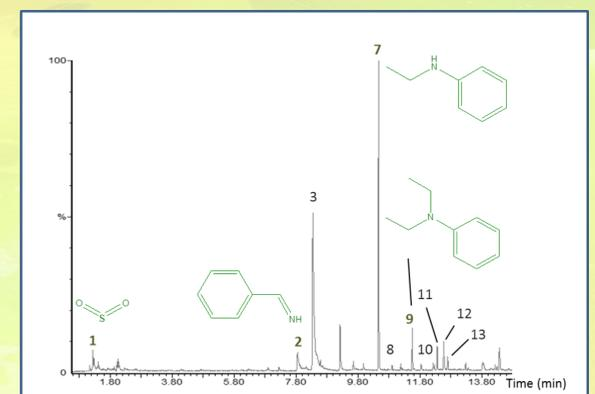
Fig. 2 Pyrogram of P1 containing light green SF yellowish dye
