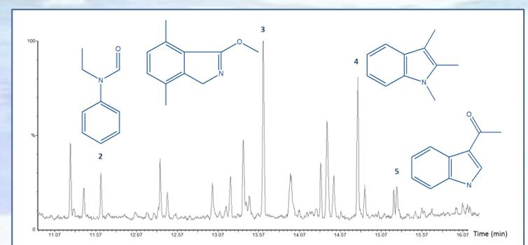
Fig. 5 Pyrogram of P13 containing carmine indigo dye
